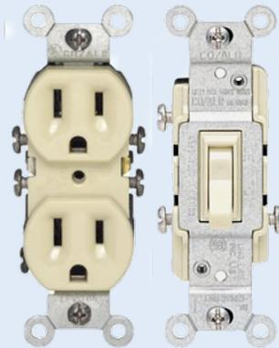
Devices with "push-in" terminations cannot be used with aluminum conductors, due to the wire's tendency to expand and contract more than copper.
